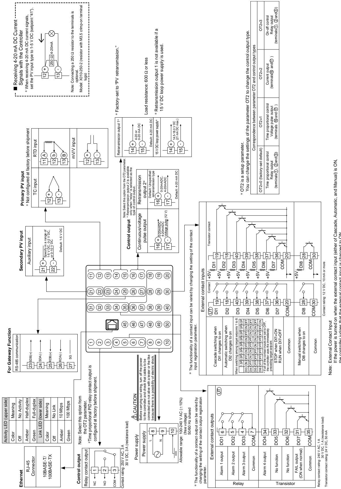
UT551 Loop Control for Backup, Terminal Arrangement
